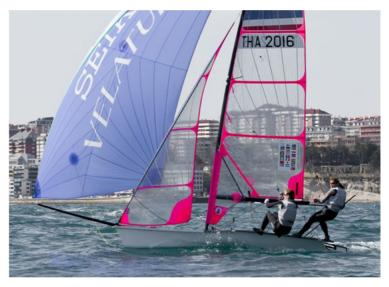
already proved to have a long lifetime with the 29er rig and a subsequent good second hand market for the hull. The boat has a low tech construction in terms of the large amount of chop strand mat and polyester used in construction, therefore the boat is relatively heavy for its size.
